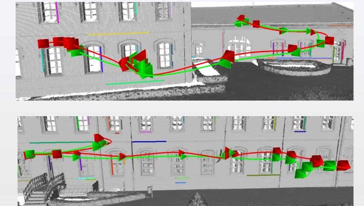
MRPnL-LM trajectory estimation results on 16 frames of a longer drone sequence. Ground truth camera poses and the trajectory are shown in green, the estimated ones in red, while the used 3D lines (81 in total) are also visible.
